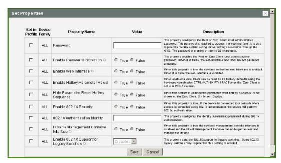
Figure 4-72: MC Security Configuration
